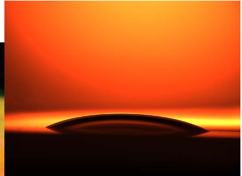
"Water droplet in oil on glass surface" by Guro Aspenes, SINTEF Petroleum Research, Bergen, Norway.
